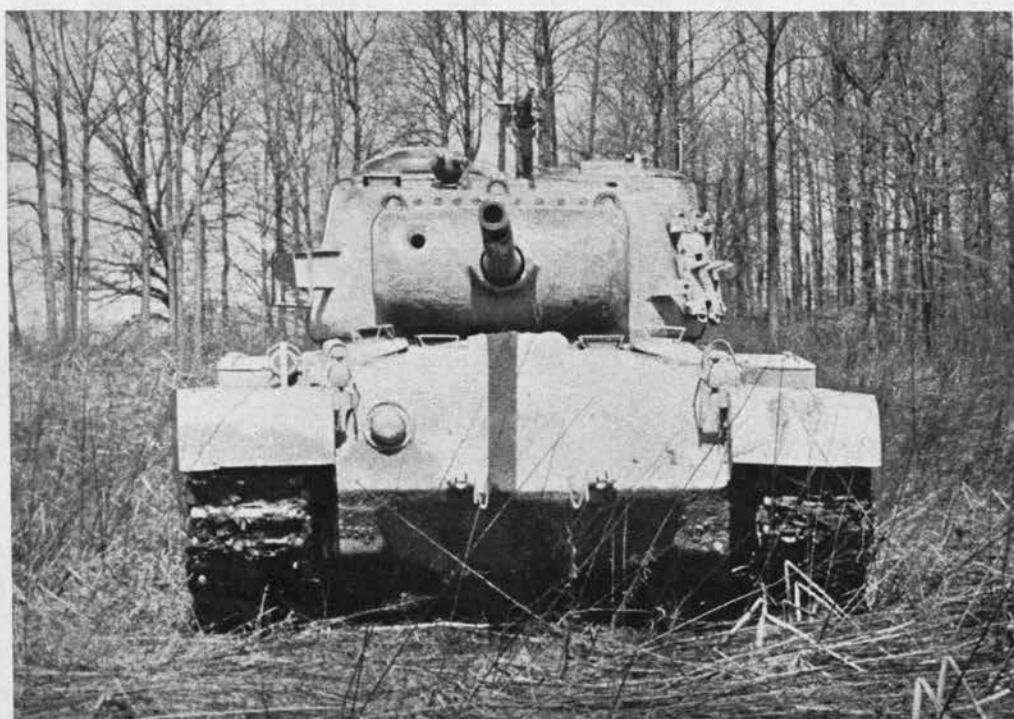
Vision cupola is at the right, the .50-caliber AA MG at dead center on the M-26's big turret. For traveling the turret is turned to the rear. Hull is set very low between massive tracks.
